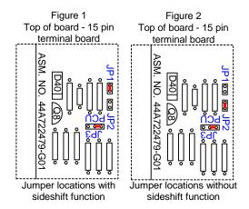
When IC3645TMM10A is supplied by the factory, it will include two small black jumpers installed on the board at JP1 and JP3, as indicated in Figure 1 above. The jumper located at JP1 enables the use of the side shift function.
